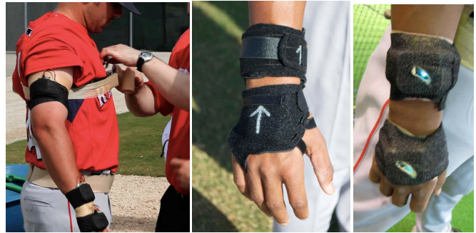
Figure 2. Attaching the Sportsemble nodes to baseball players. The nodes sit in custom Neoprene straps (center) that are taped over with Sports Wrap (left) to form a firm attachment (right).
